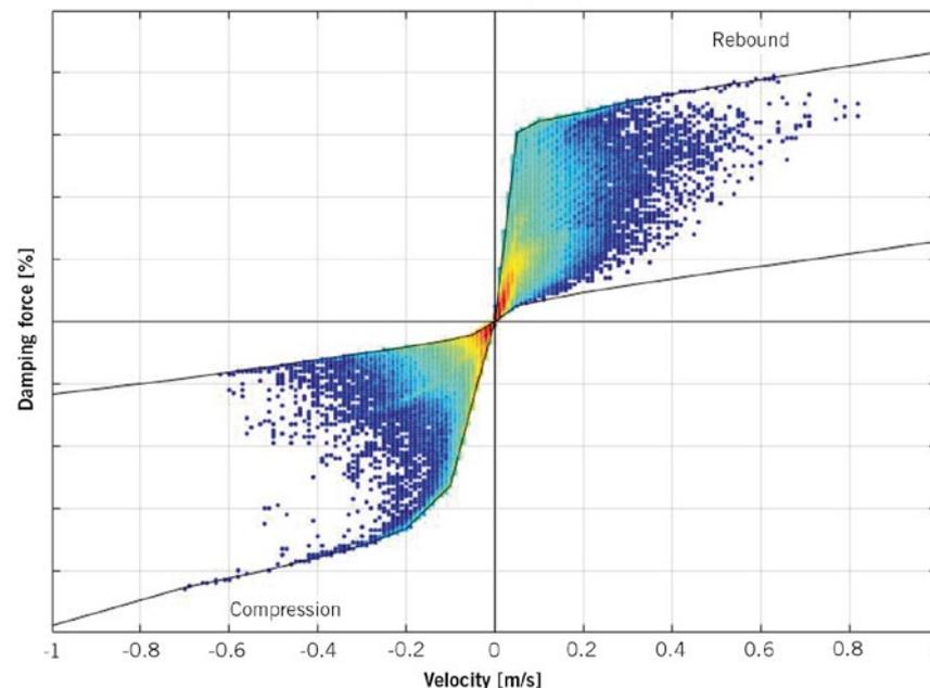
3 Use of the damping map for dynamic highway riding (top: fork; bottom: shock absorber) (© KTM)
