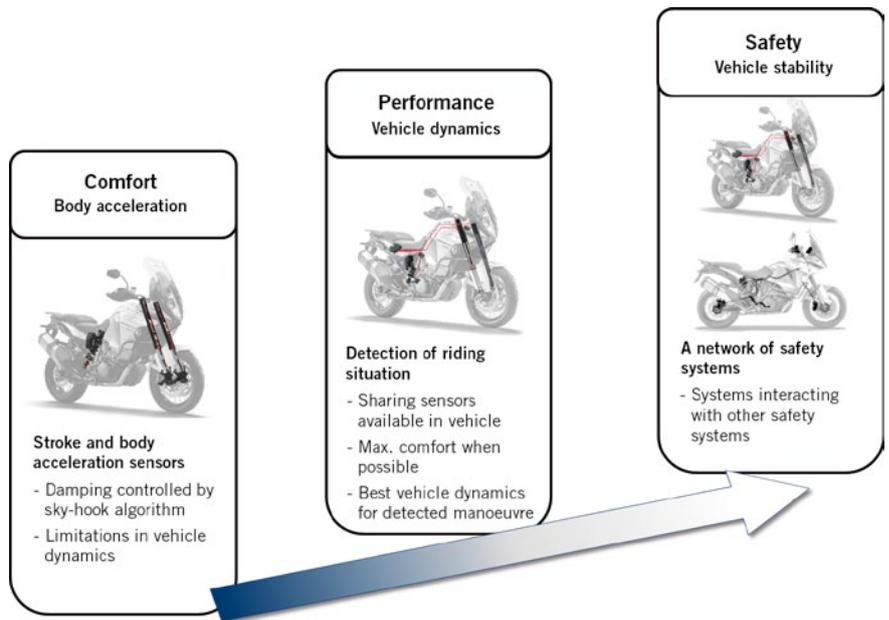
4 Stages of development for semi-active suspension in conjunction with the entire vehicle (© KTM | pictures Mitterbauer)
