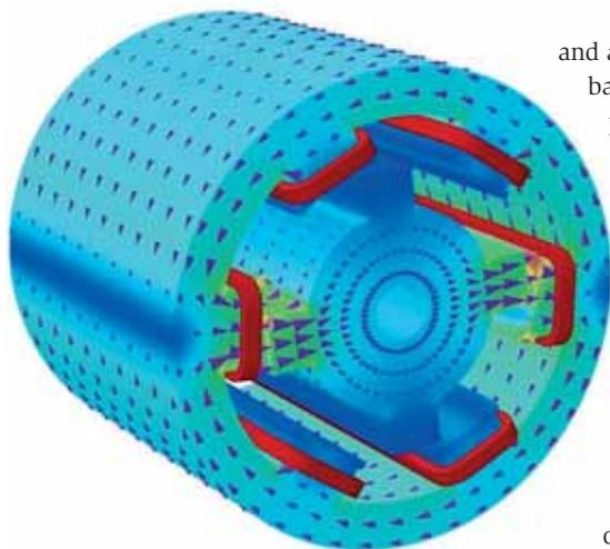
Opera's electromagnetic simulation capabilities for switched reluctance motors
