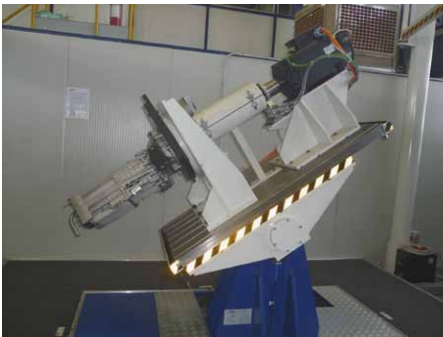
5 Lubrication verification at all attitudes with a rock-and-roll rig
