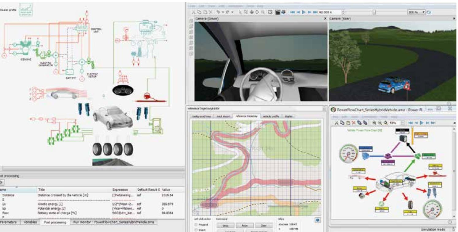
The solution also enables the handling of hydraulic and pneumatic systems for cars, trucks, buses, off-highway vehicles and trains. The multi-domain approach allows you to study evolved brake pedal amplification systems, regenerative braking and electric parking brakes. Complete ESC system template models significantly reduce modeling efforts for real-time simulation while addressing ESC homologation and combining ESC with regenerative brakes.
